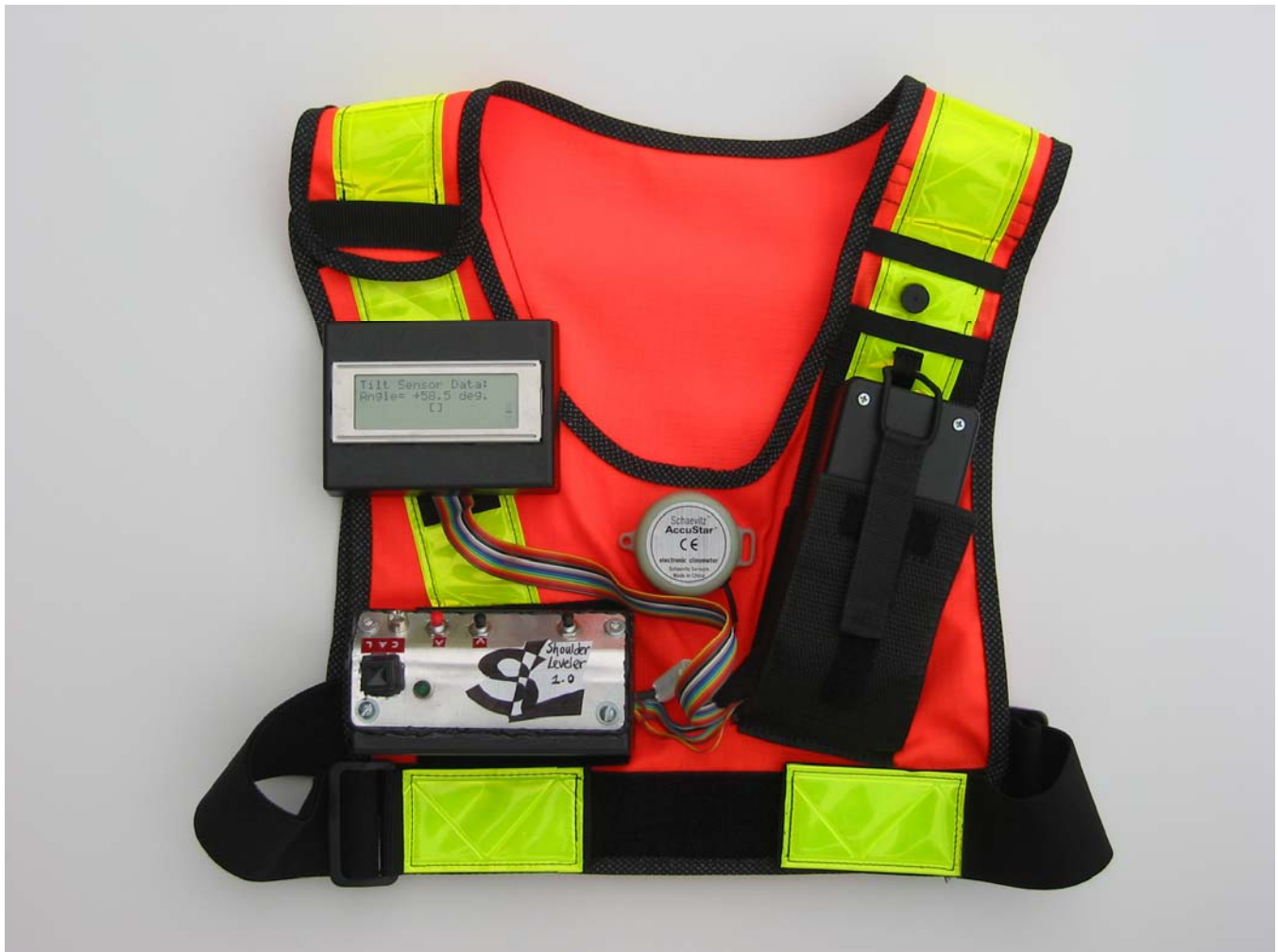
Figure 9.16. Completed Shoulder Tilt Indicator
